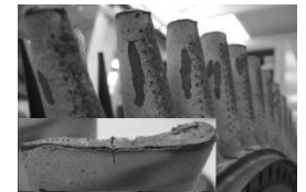
Fig. 9 Erosion of HPT vanes, [5].
