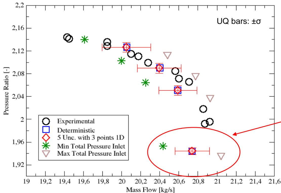
Variation of total inlet pressure modifies the choke mass flow
